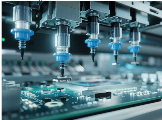
Figura 12 - Nozzles da Pick and Place
